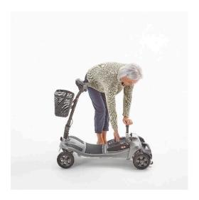
Insert the battery pack into the floorpan. Push down to ensure it is secured.
