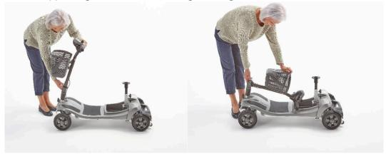
Lift up the tiller by first loosening the tiller adjustment knob and then slowly lifting the tiller up away from the floorpan. Once the tiller is upright then tighten the tiller adjustment knob to keep it in place.
