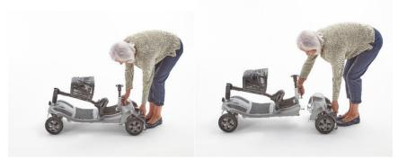
Lift up the rear section removal handle with one hand and pull down the rear section with the handle to separate the front and rear sections. Lift up and away the front section.
