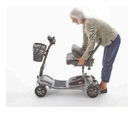
Slide the seat on to the seat post. Always check and ensure the seat is secure before sitting on the device.
