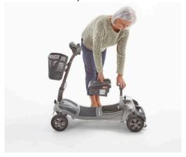
Using the handle on the battery lift up to remove the battery pack. Be aware the battery is secured in place with Velcro so if you are struggling to remove it push down on the seat post to help make it easier.
