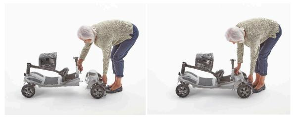
Use one hand to pull down the rear section with the handle and lift the front section using either the seat post or rear section removal handle. Drop the front section into the rear section and push down until you hear a click. Always check that the sections are connected correctly before moving on to the next stage.
