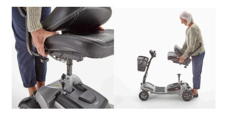
Lift up the seat rotation lever and lift the seat upwards to remove it.
