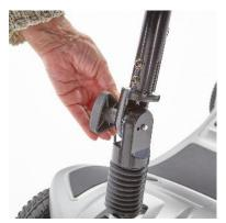
To adjust the tiller, hold the tiller in one hand and turn the tiller adjustment knob anti clockwise with the other until the teeth disengage and the tiller can move up and down freely.
