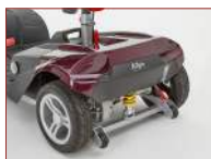
Rear monoshock suspension
